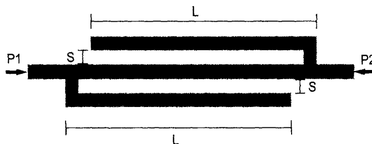
Figure 10.16: Double-folded microstrip stub bandstop filter
