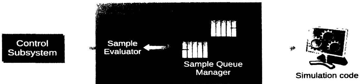
Figure 4.13: The sample queue manager forms the bridge between the control subsystem and the sample evaluation backend.
